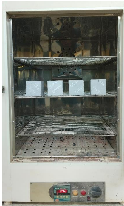
Figure. 5 Specimens cured in Hot Air Oven
