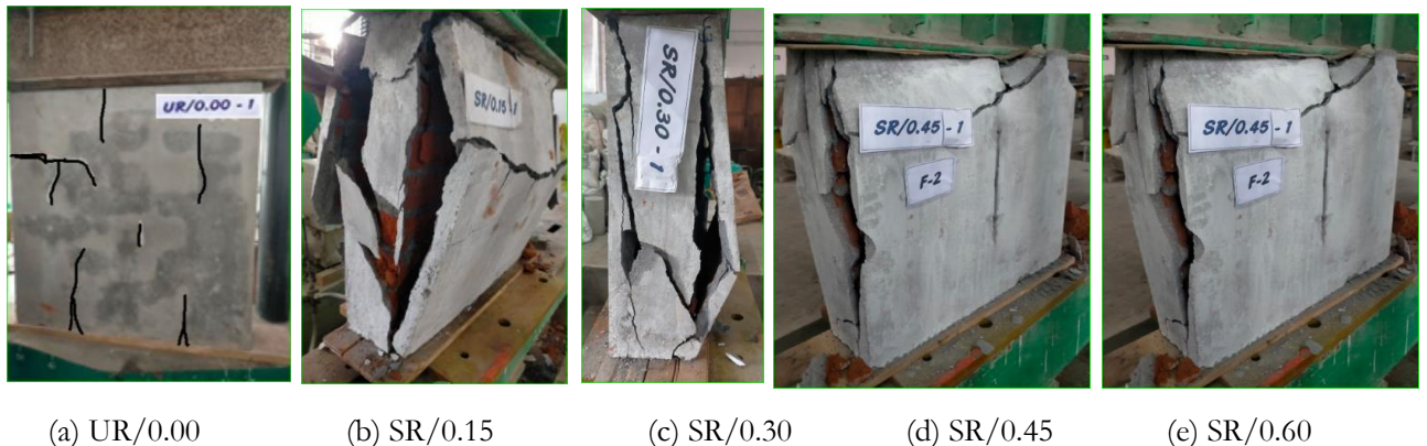
Figure 3 Crack pattern in compression specimens
