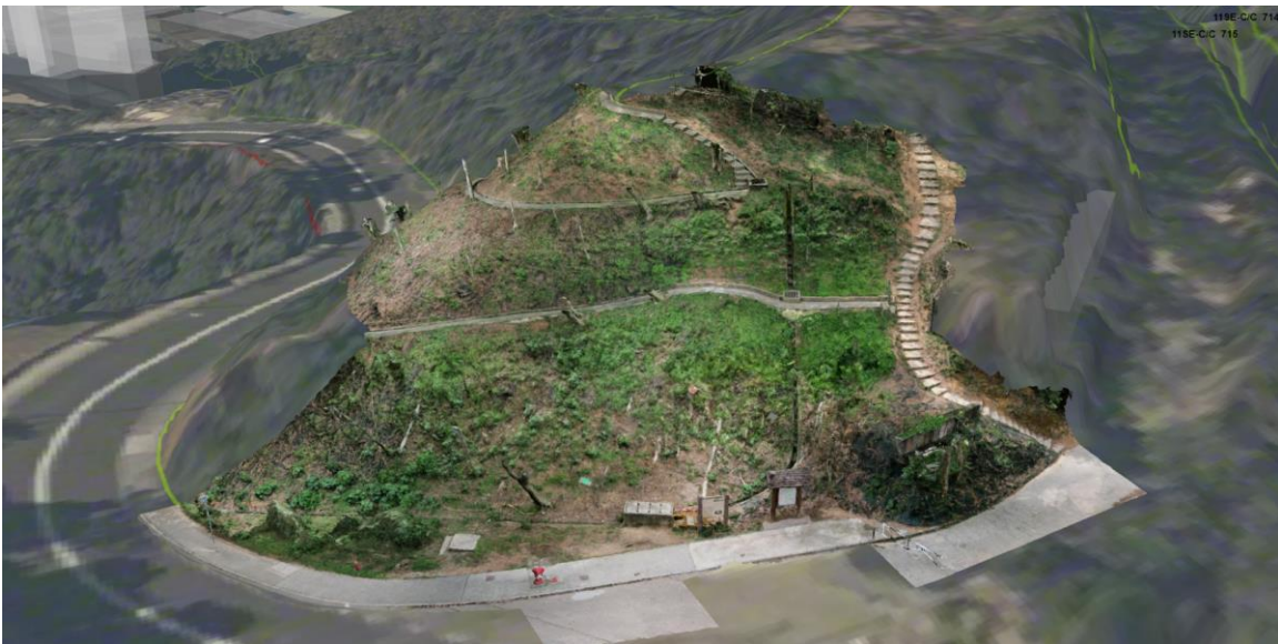
Figure 8: Photorealistic 3D mesh model of 11SE-C/C717 at Tai Tam Reservoir Road that is superimposed to the terrain based on aerial photographs
