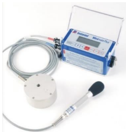
Plate 1: Vibration Sensor with Automatic Remote Data Transmission
