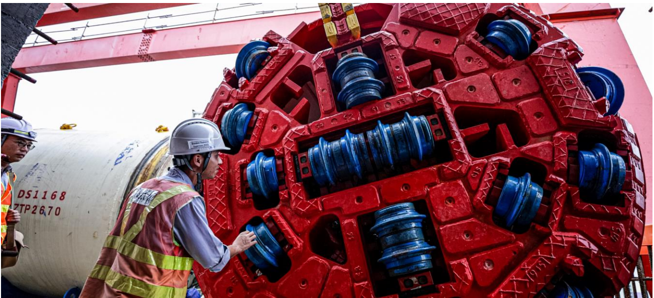
Photo 4 – Adopted cutter head for hard rock MTBM
