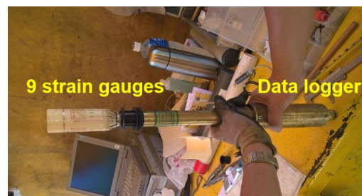
Figure 14a & 14b: Pilot concentric hole (left) and triaxial measuring cell (right)
