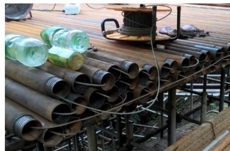
Figure 6a & 6b: OTV tool in end of drill string (left) and cable threaded through 1km long drill rod (right) for HDC
