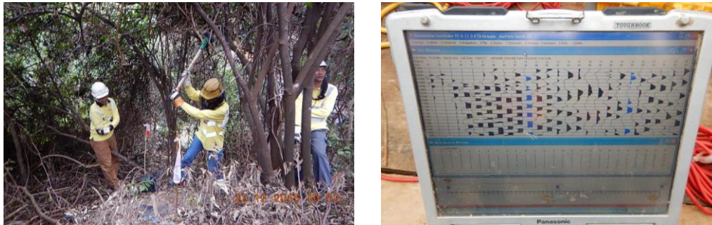
Figure 7a & 7b: Hammer hitting along the seismic lines (left) and signals analysis (right)
