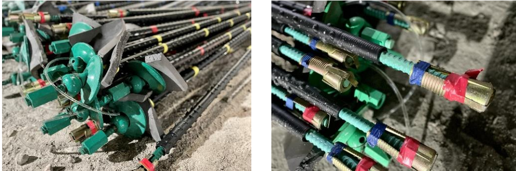
Figure 23a & 23b: Permanent rock bolts with specific corrosion protection (left) and expansion shell at end (right)
