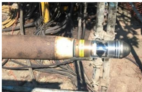
Figure 6a & 6b: OTV tool in end of drill string (left) and cable threaded through 1km long drill rod (right) for HDC
