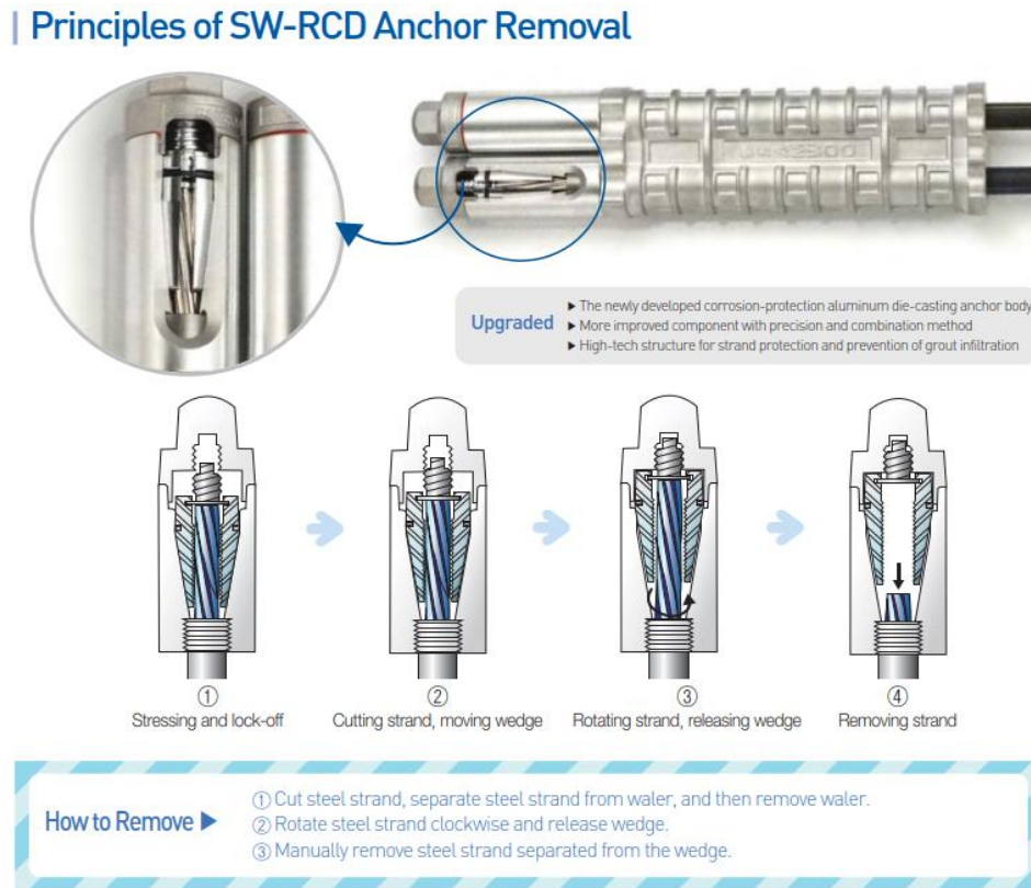
Figure 8: Principles of Removing SW-RCD Anchors (SAMWOO)
