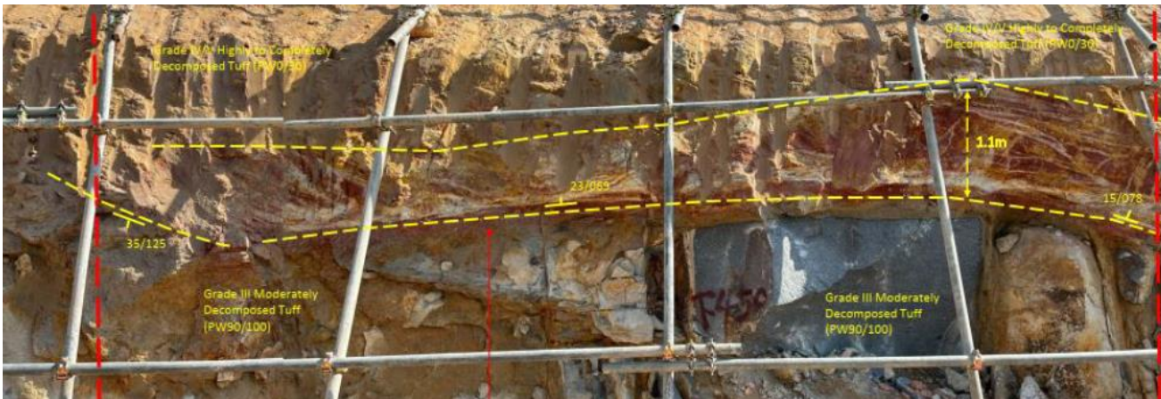
Plate 3: Thin veins or stringer of white, firm sandy clay occurs sub-parallel to the surface of grade II/III rock
