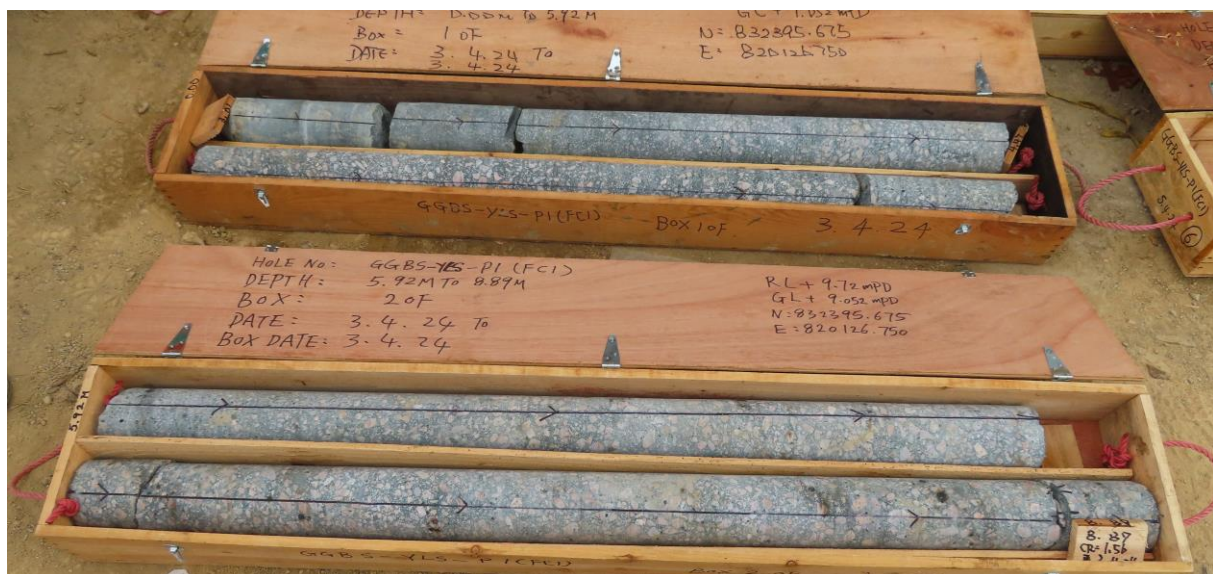
Figure 3.4: Full-length concrete core drilled from GGBS-YLS-P1 after 28 days of concreting
