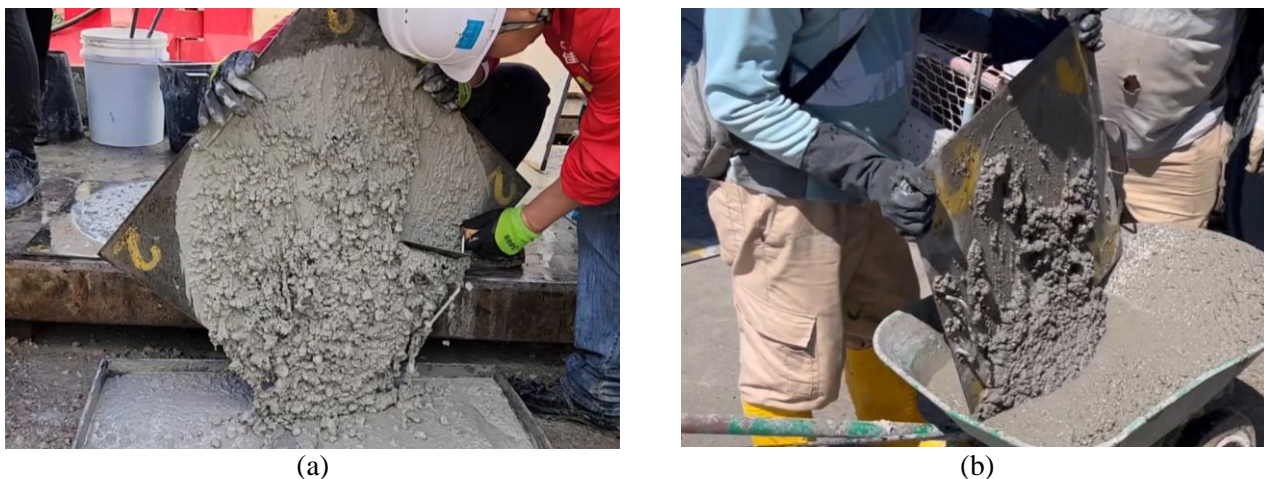
Figure 3.1: Different degrees of adhesiveness of concrete observed during slump tests: (a) 80% GGBS (GGBS-YLS-P2); (b) PFA concrete (observed at another site)
