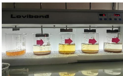
Figure1: Leachate treatment by chemical coagulation/ flocculation
