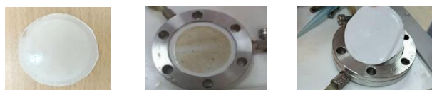
Figure 2. Photograph of the PVDF membrane in a filtration system before and after clogging (view of the active surface and the underside)
