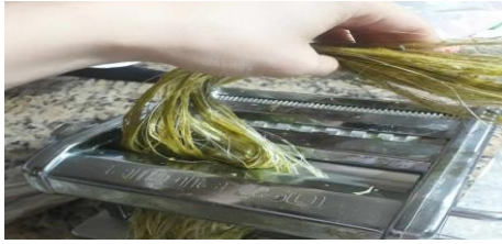
Figure 1: Mechanical fibre extraction
