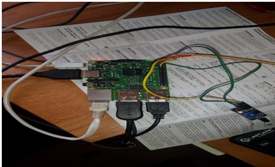
Fig 5.1: Raspberry Pi containing wireless PIR and fire detection sensor.
