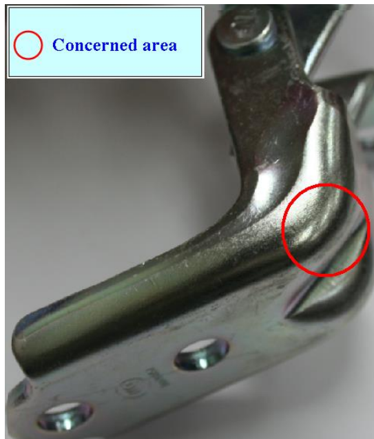
Figure 3.10: Case No. 8: R=20\text{mm} , a=20^\circ , b=90^\circ , r=5\text{mm} , I=0.748 . No crack occurred in concerned area
