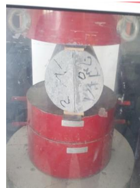
Figure 4: Splitting tensile test set-up.
