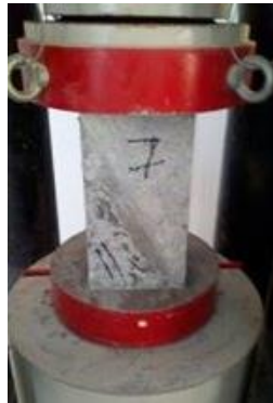
Figure 3: Slant shear test set-up.
