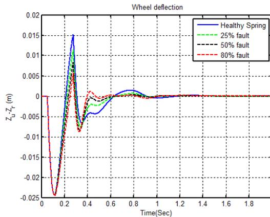
**Figure 6** *Wheel deflections for different spring stiffness*
