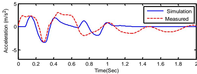
**Figure 3** *Vibration (acceleration) of suspension simulation and experimental*
