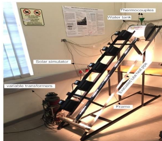
Figure 3: The heat pipe’s testing apparatus
