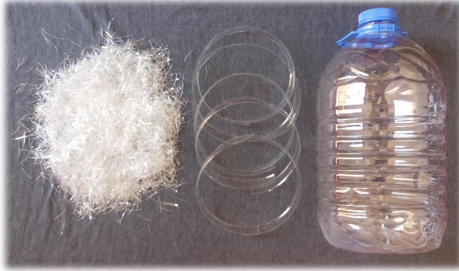
Figure 1: Preparing of PET from plastic bottles
