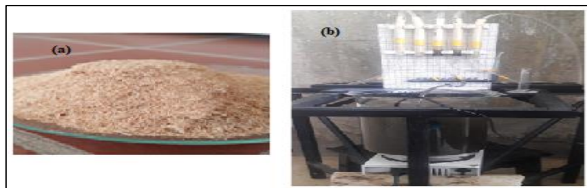
Figure 1: a): Crashed date pedicels; (b): Experimental setup designed for column tests
