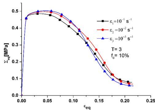
Figure 1: Equivalent stress as a function of equivalent strain at different strain rates.
