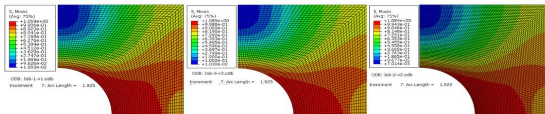
Figure 2: illustrates the Isovalues of maximum equivalent stresses at the cavity coalescence point.
