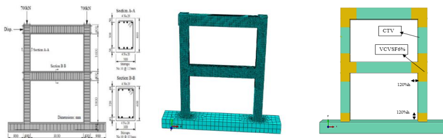
Figure 1: Modeling of the frame using the Abaqus code.
