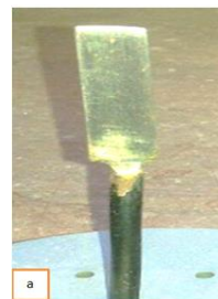
Figure (5): Coated sample of mild steel immersed in sea water for 5 days
