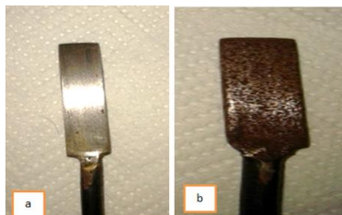
Figure (4): Uncoated sample of mild steel immersed in sea water for 5 days
