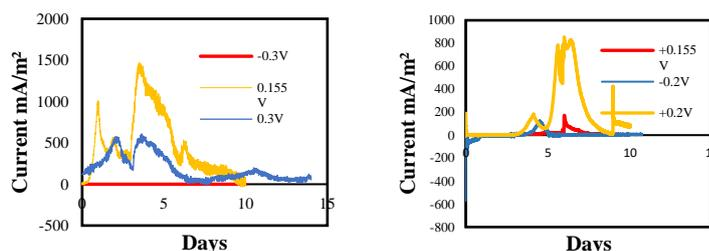
Fig. 1 Chronoamperometry of a) soil and b) sediment at different potentials
