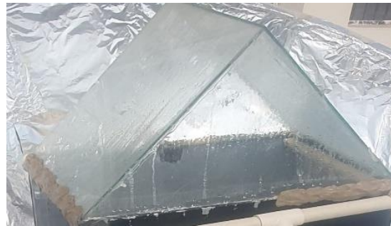
Figure 8: Double Slope Glass
