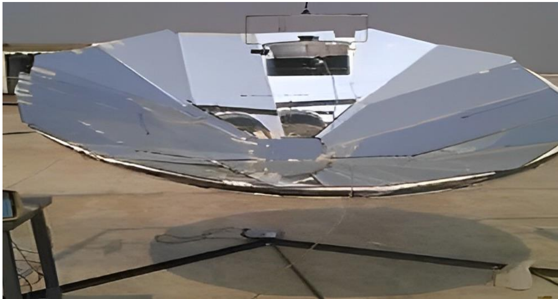
Figure 2: Stainless Steel as a Reflective Material
