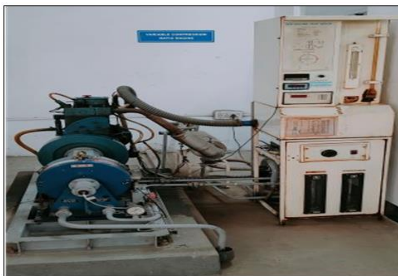
Figure 1: VCR engine and testing setup
