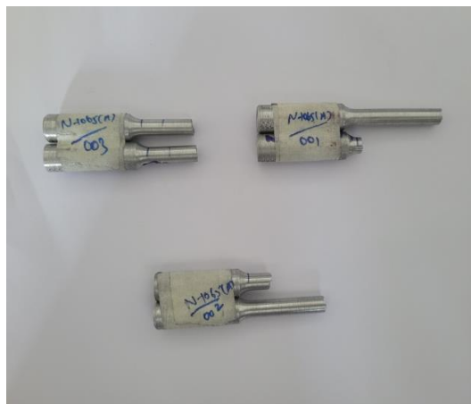
Figure 5: Tensile test Specimen
