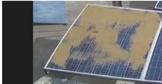
Figure 12(a): Result obtained from ML model (Fault (Dust accumulation)- Hardware result)
