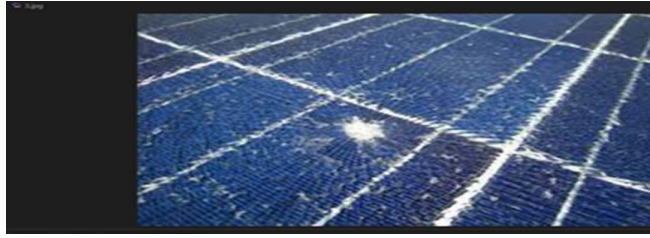
Figure 11(a): Result obtained from ML model (Fault (Cracks)- Hardware result)
