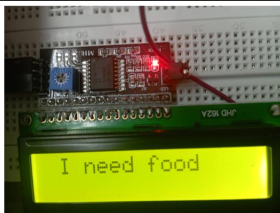
Figure 4: Food Requirement of Patient displayed in LCD
