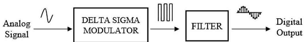
Figure 1: Schematic model of Delta Sigma A/D Converter
