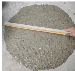
Figure 4: Flow spread of SCC
