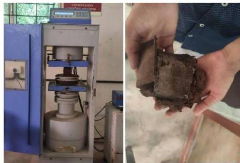
Figure 8: Test setup and specimen failed in compression.
