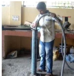
**Figure 3:** Casting of specimen using needle vibrator
