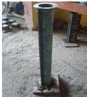
**Figure 1: Mould fixed on base plate**
