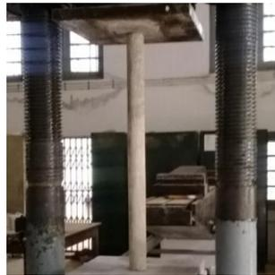
**Figure 6:** *Axial load test setup*
