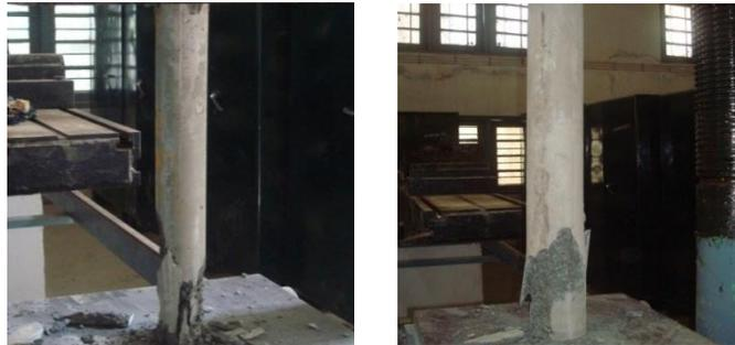
**Figure 8:** Specimens with failure at the ends
