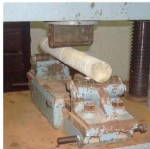
**Figure 7:** *Bending test setup*
