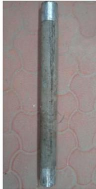
**Figure 5:** *Specimen cast with end sleeves*
