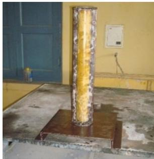
**Figure 2:** Casting of specimen using vibration table
