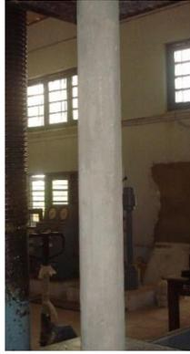
**Figure 4:** *Specimen cast without end sleeves*
