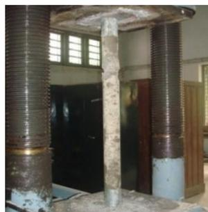
**Figure 9:** Specimen with failure away from the ends due to end sleeves
