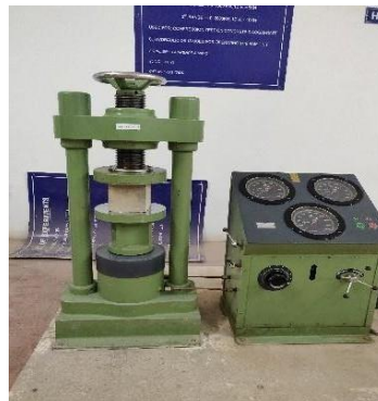
Figure 2: Compression testing of cube specimen
