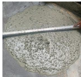
b) Slump flow test
