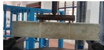
c) Flexural strength- crack on the beam
