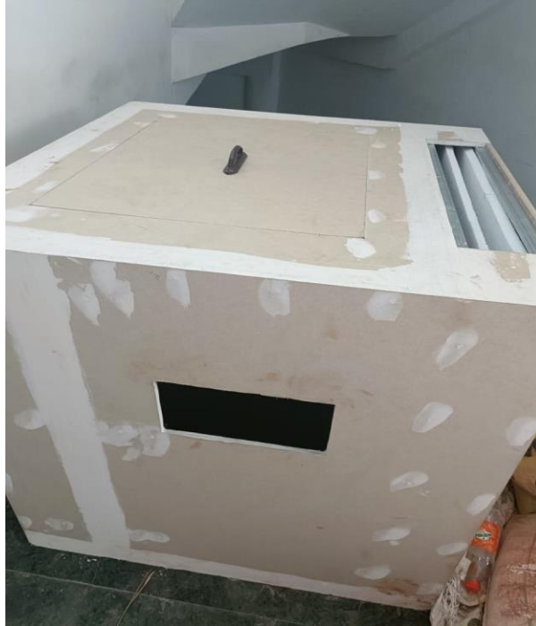
Figure 10: Scenario 3 - With EPS sheets- two layer in the centre of gypsum partition wall
