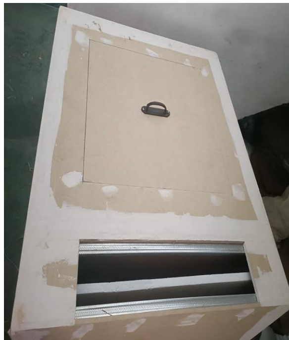
Figure 9: Scenario 2 - With EPS sheet -one layer in the centre of gypsum partition wall
