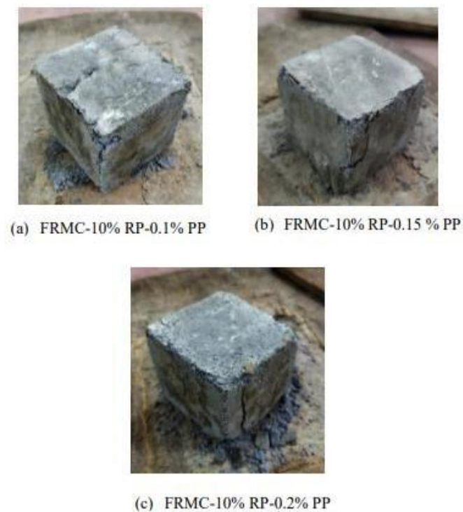
Figure 11: Failure mode of mortar cubes with polypropylene fibers
