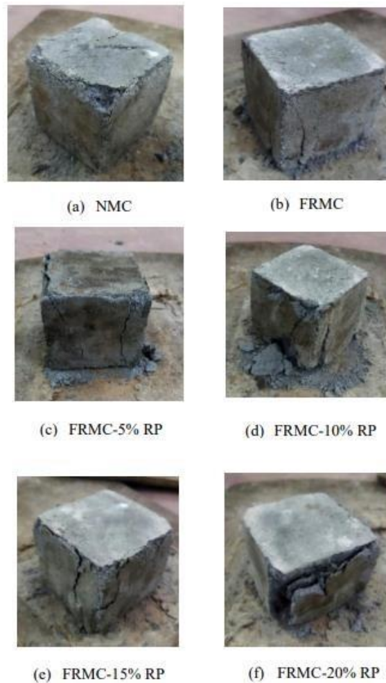
Figure 9: Failure mode of mortar cubes
