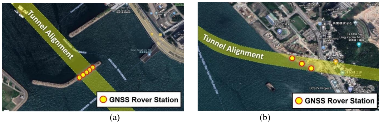
Figure 3: (a) Phase 2 GNSS monitoring: at Kwun Tong Typhoon Shelter breakwater and (b) along Cha Kwo Ling seawall
