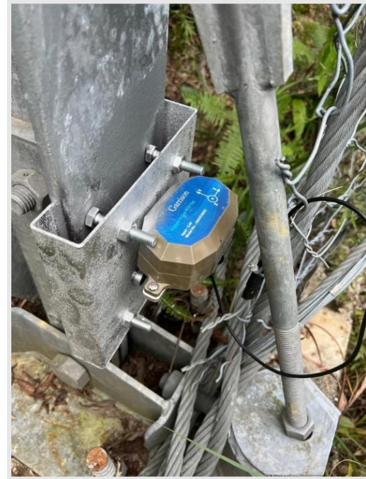
Figure 7: Schematic Details of Steel Clamp for Sensor Fixing Figure 8: Photo of Sensor Fixing to Steel Post
