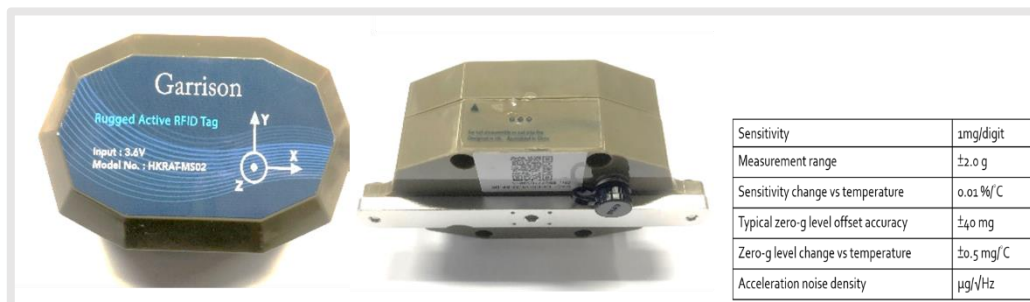
Figure 3: Tailor-made IoT Sensor
