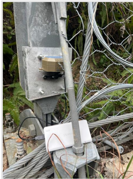
Figure 9: Photo of Sensor Charging using power bank
