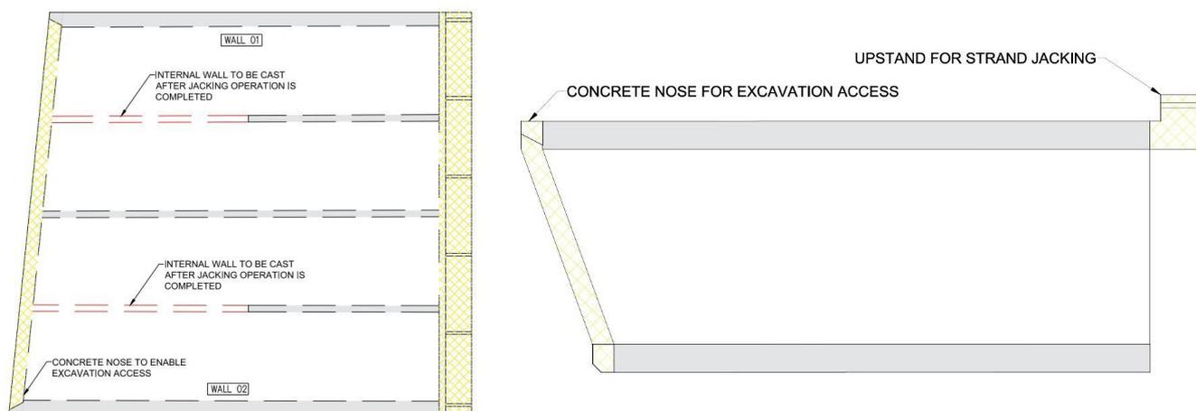
**Figure 14:** Plan View and elevation of APM & BHS Boxes
