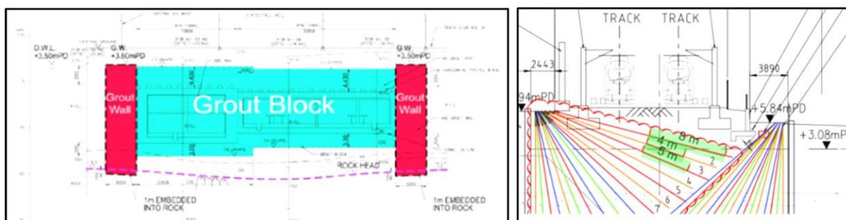
Figure 19: a) Cross section Grout Walls and GBUAEL; b) Typical Fan Grouting Section under AEL
