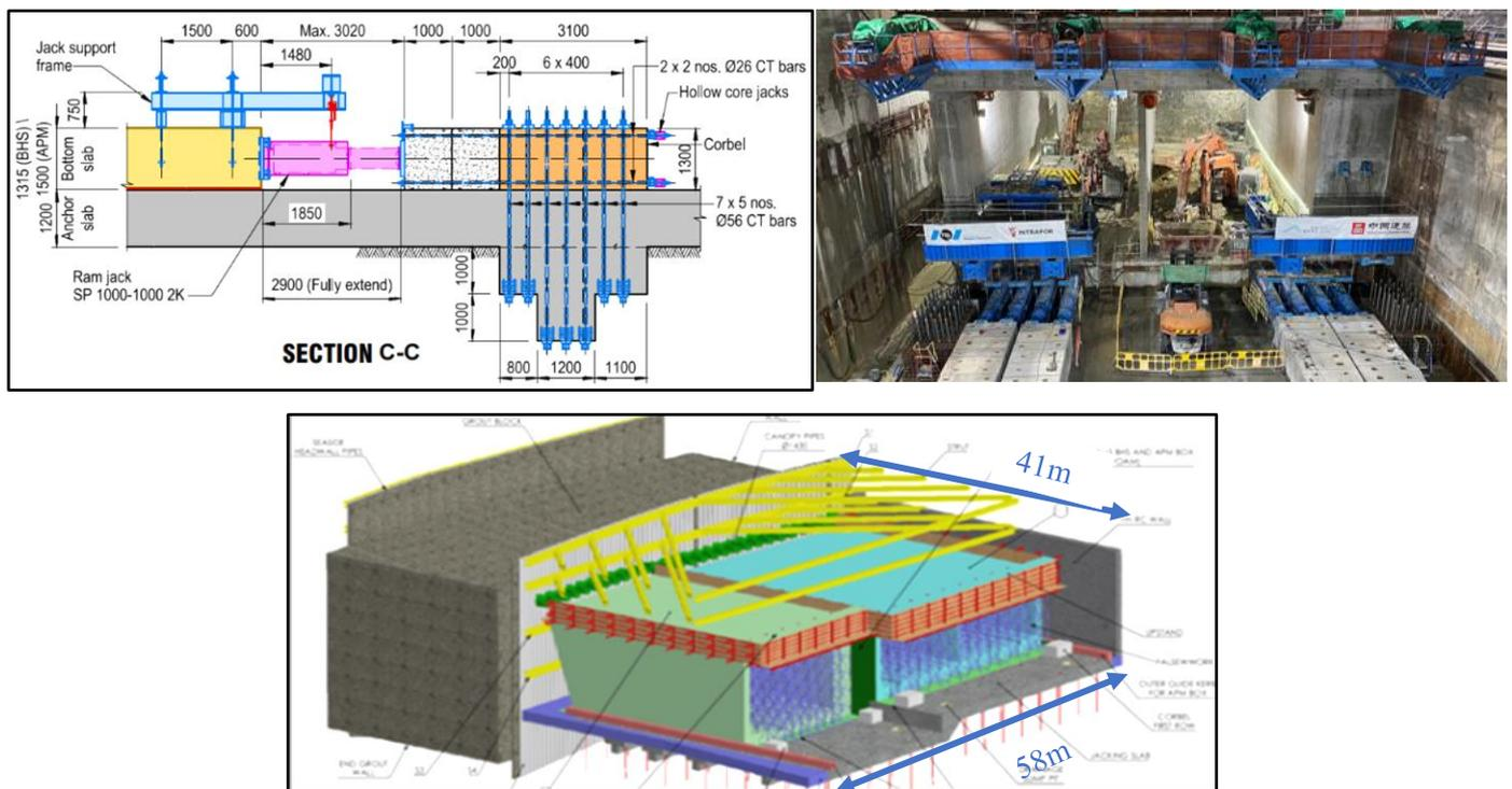
**Figure 21:** Construction of APM and BHS Tunnel Boxes in Jacking Shaft on top of Jacking Slab
