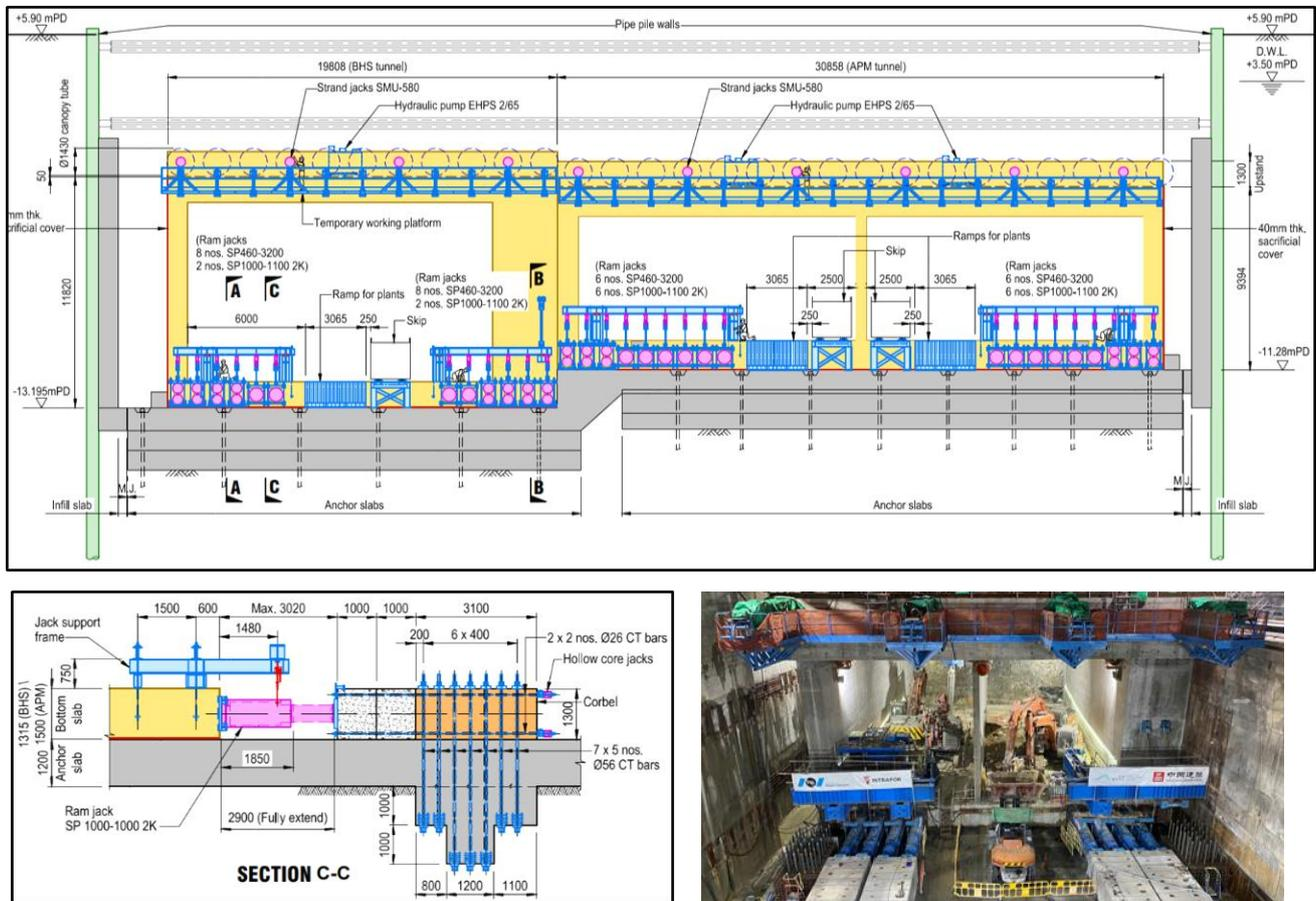
Figure 23: Typical Arrangement of push jacks at rear of APM and BHS box
