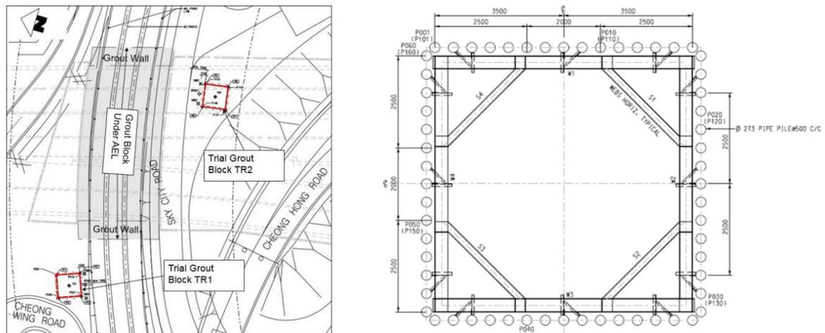
Figure 17: Location and cofferdam of Grout Trial Block (GTRB) TR1 and T2
