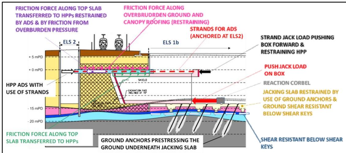
Figure 28: Load path during box jacking
