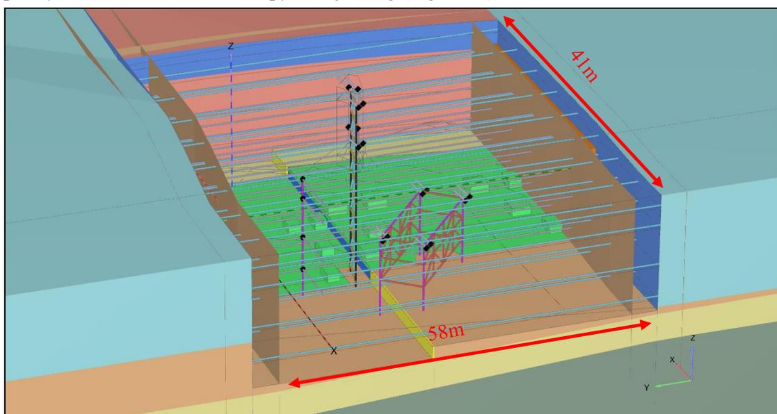
Figure 25: Plaxis 3-D model for the analysis of the jacking slab
