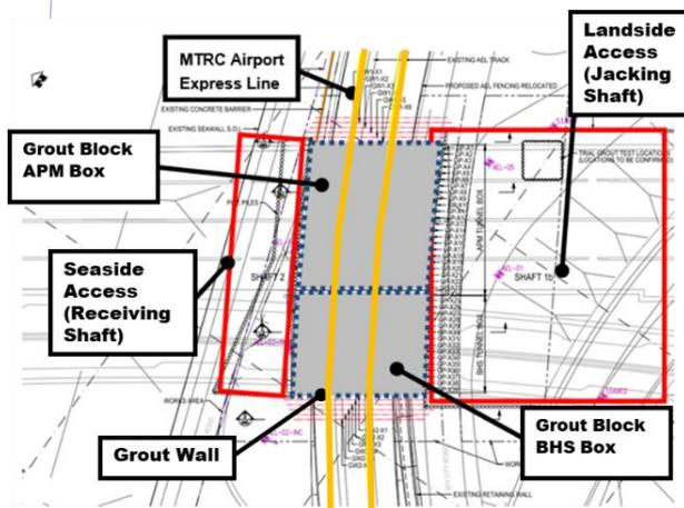
Figure 15: Footprint of Receiving and Jacking Shafts
