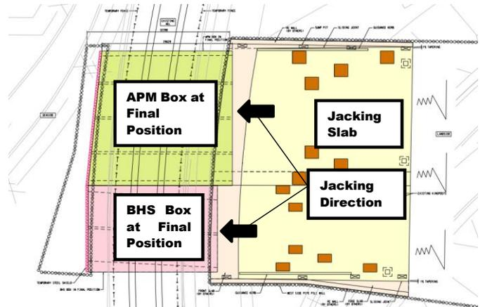
Figure 16: General Plan of Box Jacking Works
