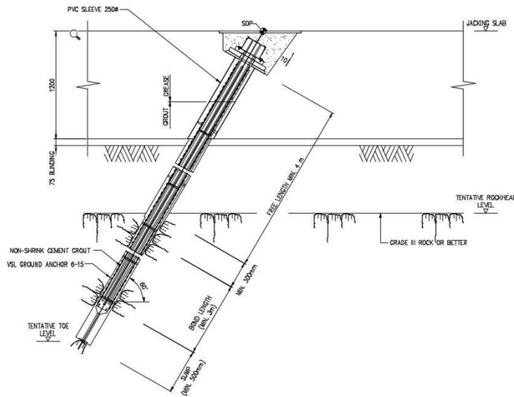
Figure 27: Typical Arrangement of Inclined Ground Anchor
