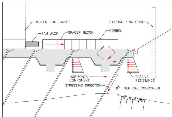
Figure 24: Jacking slab restraint load considerations
