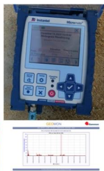
Figure 8: Real Time Vibration Monitoring for Chee on Bridge
