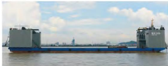
Figure 11: 15000DWT Semi-submersible Barge (ZHONG REN 1500)
