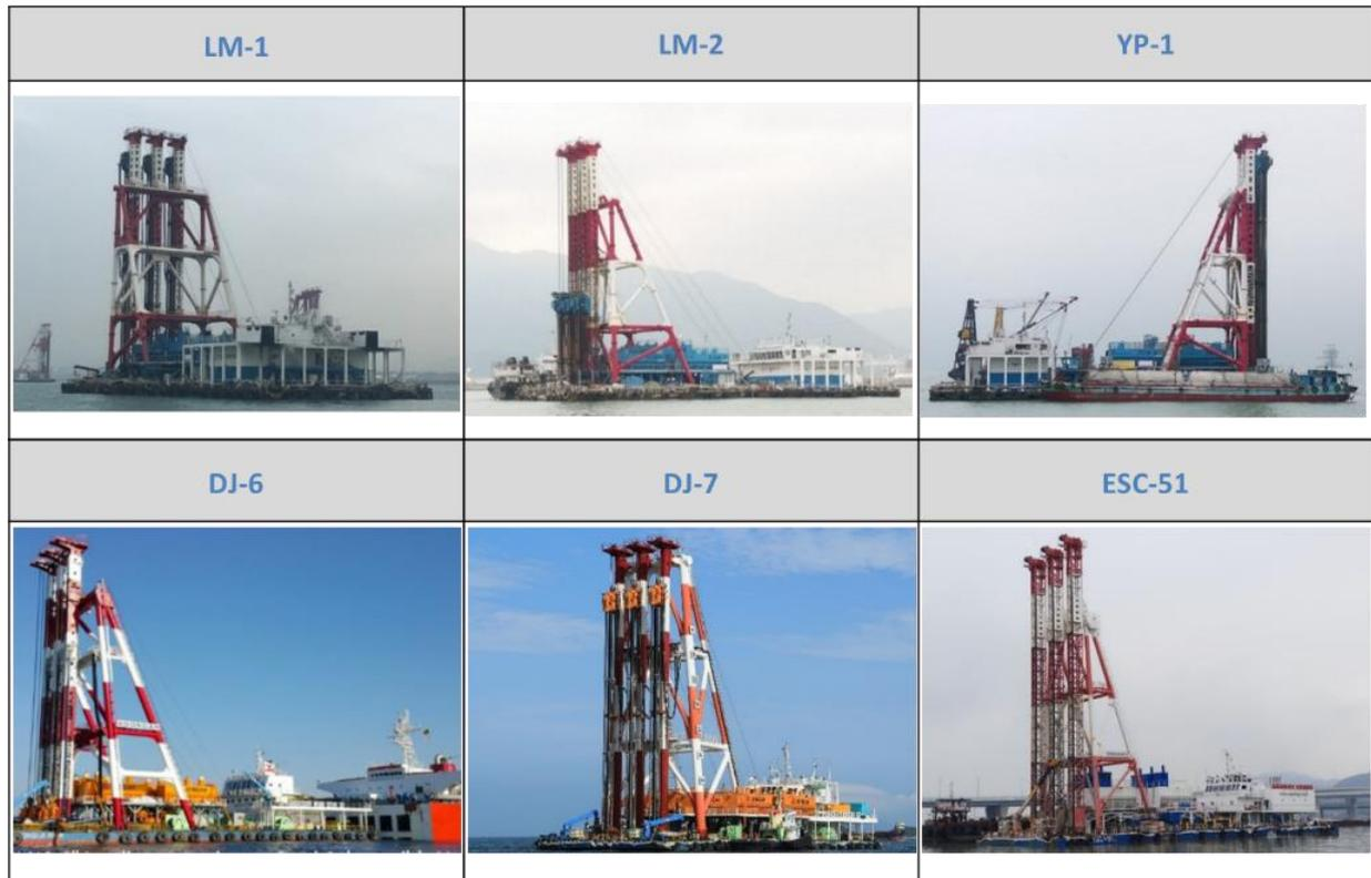
**Figure 6:** Marine DCM barges used in TCE project.
