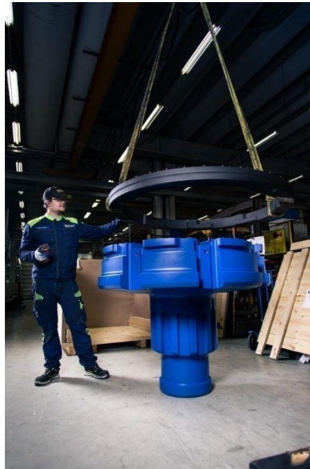
Figure 9: A large-sized Spiral Flush pilot bit
