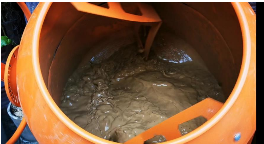
Figure 1: Step I for mixing and washing soil with water.
