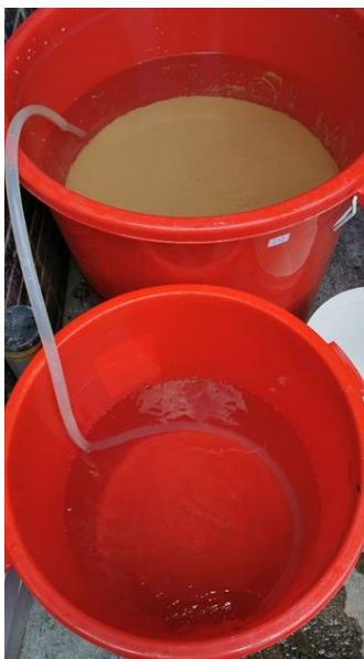
Figure 5: Step IV for recycling water from clay slurry and obtain clay material.
