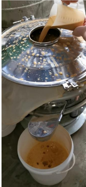
Figure 4: Step III for washing and sieving mud slurry into silt and clay slurry with water
