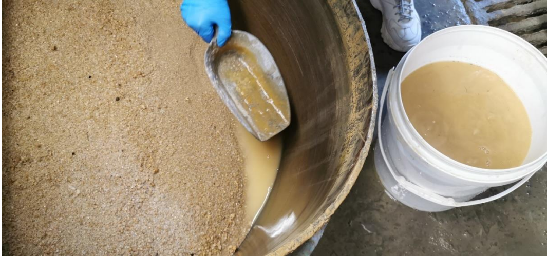
Figure 2: Results of clean sand and soil slurry from Step I of mixing and washing soil with water.
