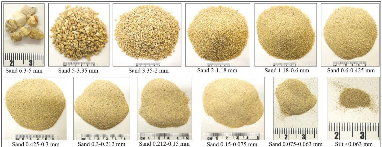
Figure 8: The 12 individual particle sizes of the CDG sand in Figure 6 by dry sieve method
