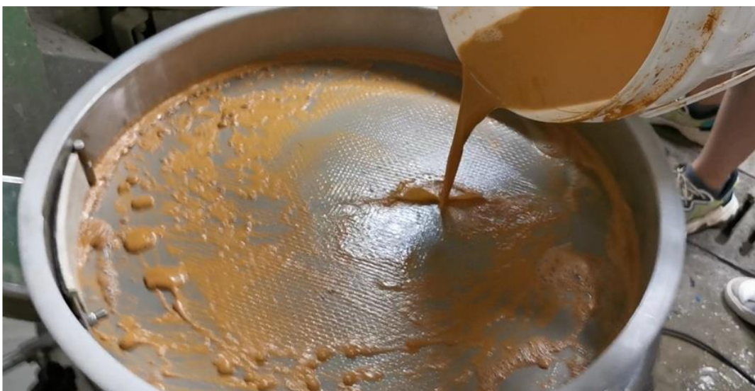
Figure 3: Step II for washing and sieving soil slurry into fine sand and mud slurry with water
