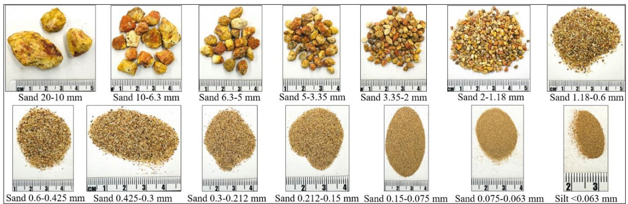
Figure 14: The 14 individual particle sizes of the CDV sand in Figure 13 by dry sieve method
