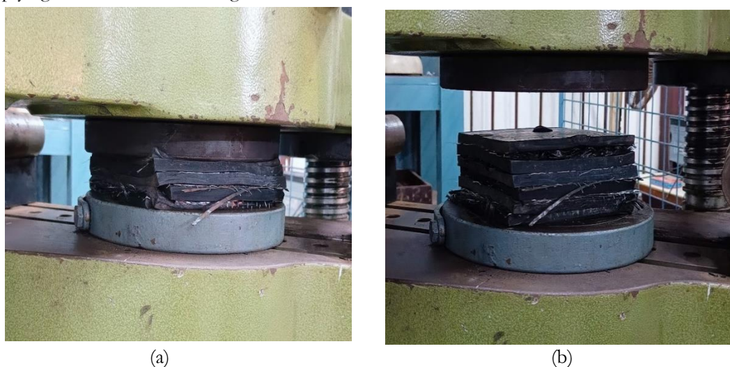
Figure 5: Isolator specimen (a) during and (b) after applying load
