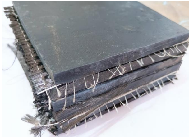
Figure 3: Base isolator specimen with CFRP
