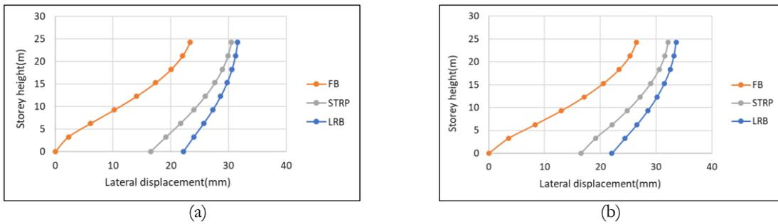
**Figure 9:** Lateral displacement of various models – (a) along X direction (b) along Y direction
