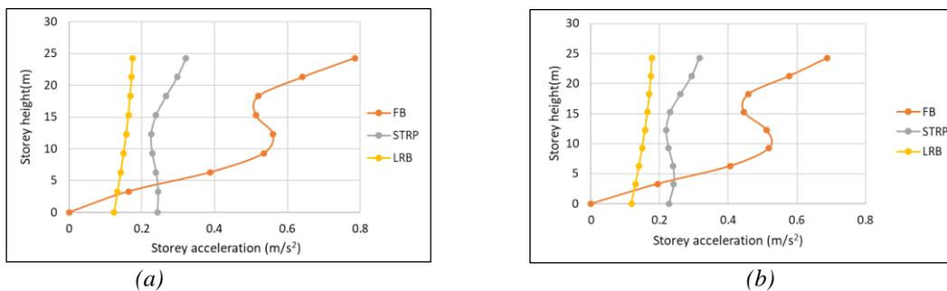
**Figure 11:** Storey acceleration of various models – (a) along X direction (b) along Y direction
