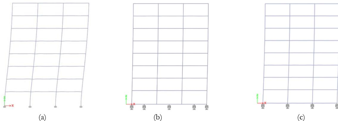
**Figure 8:** Deformed shape of models in response spectrum analysis- **(a) fixed base model**, **(b) model with STRP** and **(c) model with LRB**
