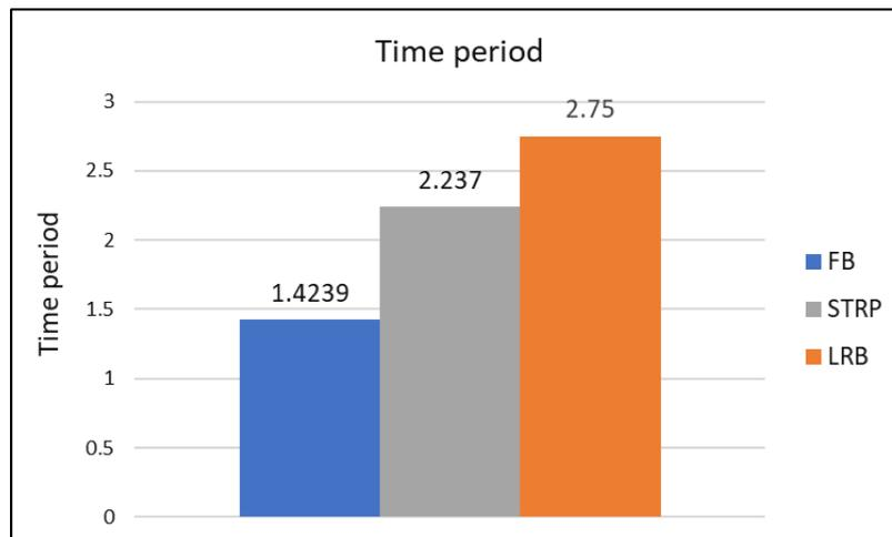
Figure 13: Enhancement of time period with base isolators
