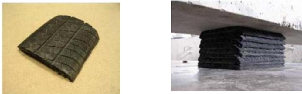
**Figure 3: (a) Scrap tyre pad, (b) Scrap tyre pad isolator: (Source: Turer et al, [10])**
