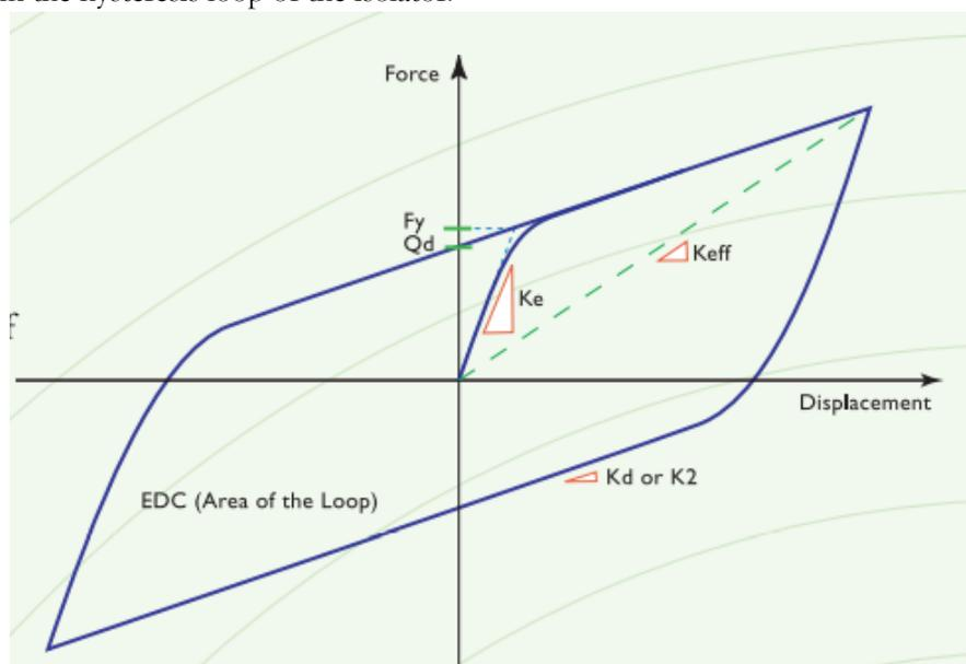
**Figure 4: Force-displacement loop of conventional isolator**
