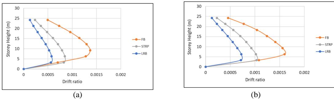
**Figure 10:** Drift ratio of various models– (a) along X direction (b) along Y direction
