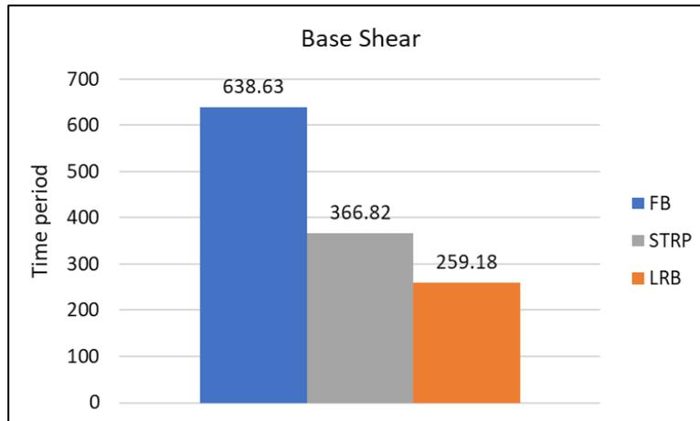
Figure 12: Reduction in base shear with STRP and LRB isolators
