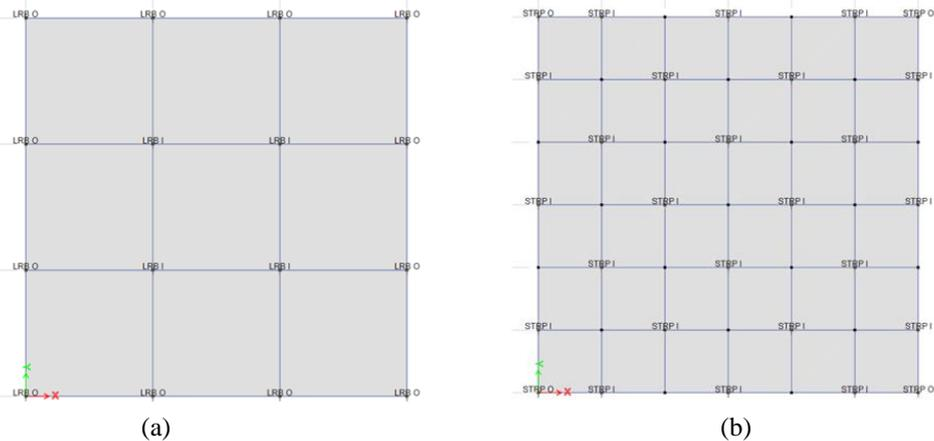
**Figure 6:** Plan of building model with (a) LRB and (b) STRP
