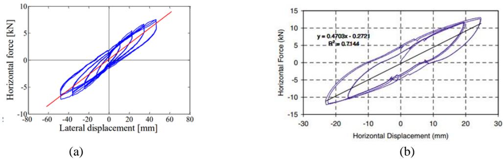
**Figure 7:** Load displacement hysteresis of STRP adopted for- **(a) Outer Isolators** [9] (Mishra et al.), **(b) Inner Isolators** (Turer et al.) [10]
