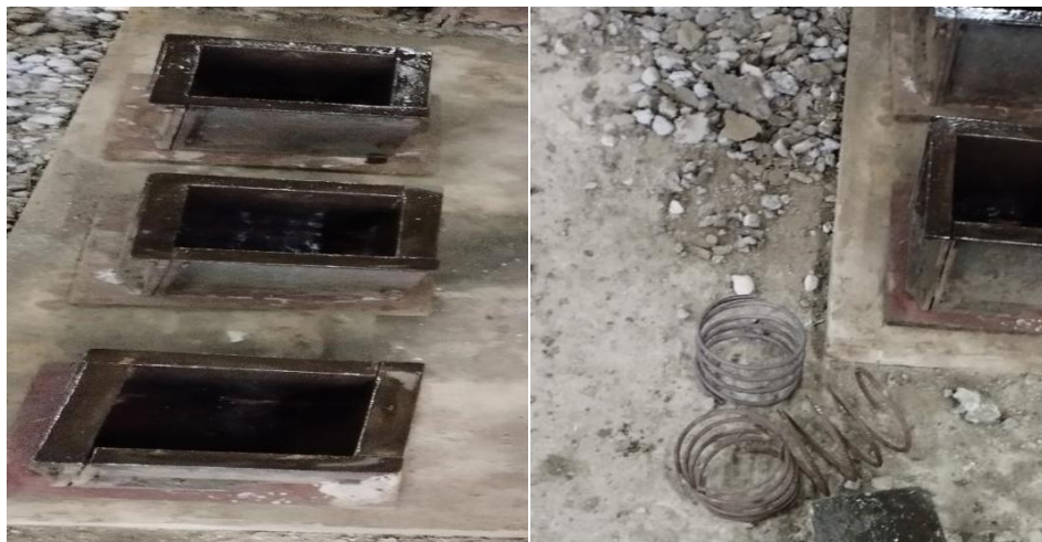
Figure 1: Mould and helical spring
