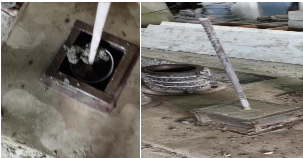
Figure 3: Inserting helical spring and sample specimen after casting.
