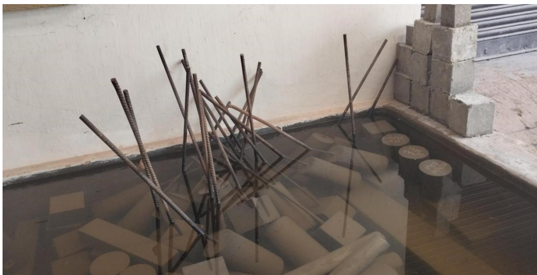
Figure 4: Curing of specimens.
