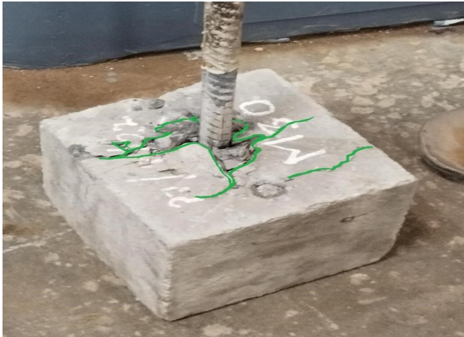
Figure 9: Failure pattern of M30
