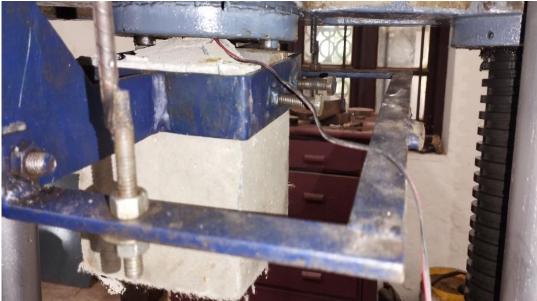
Figure 13: Failure of ECC specimen
