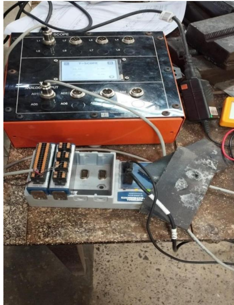
Figure 7: T-SCOPE (Data acquisition system)
