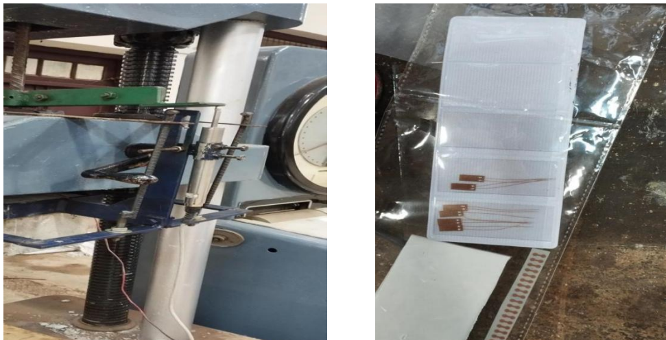
Figure 6: LVDT and strain gauge
