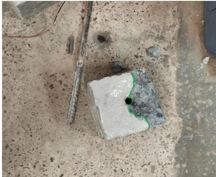
Figure 11: Failure pattern of GPC
