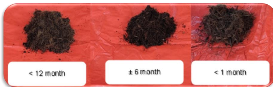
Figure 3: Grading shell based on the age of the waste.
