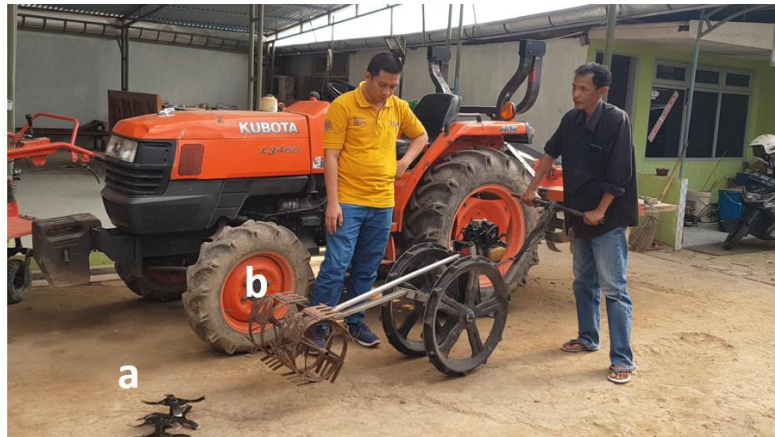
Figure 8. Multifunction rice weeding tool with different features: (a) soil block material mix and (b) weeding activity
