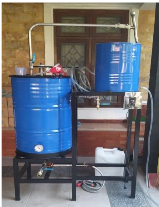
Figure 5: Used cooking oil diversification reactor with a capacity of 100 L
